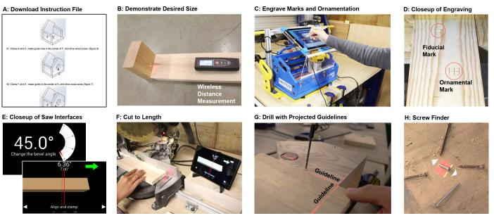
Figure 2: To complete a Drill Sergeant project, a user finds a model (a) and sizes it, measuring their desired final location (b). For this birdhouse, the user engraves a decorative pattern and fiducials (c, d), cuts boards to length (e, f), locates drill positions (g), and identifies the correct fasteners (h).
