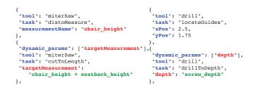
**Figure 4:** Our JSON-based language has dynamic and static parameters for instructions; formulas are evaluated in Python. This language captures all tasks, from measuring a dimension and cutting to length on a saw (left) to locating and drilling in the correct location (right).
